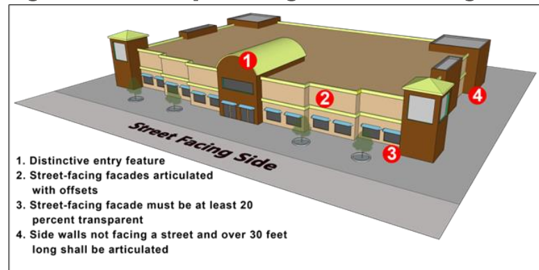
Figure II-17: Example of “Big Box” Store Design
