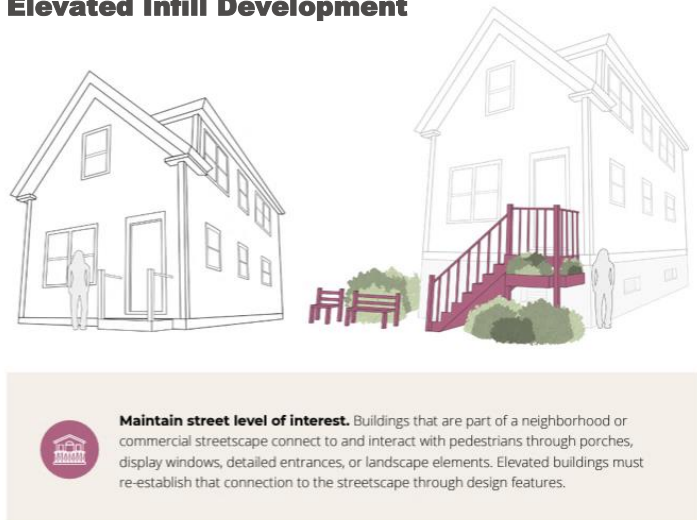
Figure II-13. Example Design Standards for Elevated Infill Development
