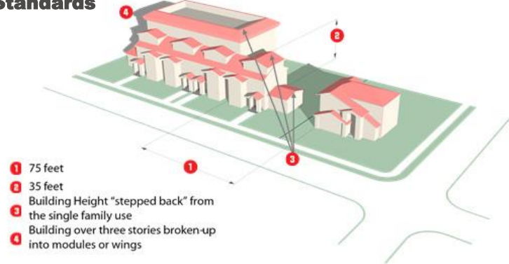
Figure II-18: Sample Building Height Compatibility Standards
